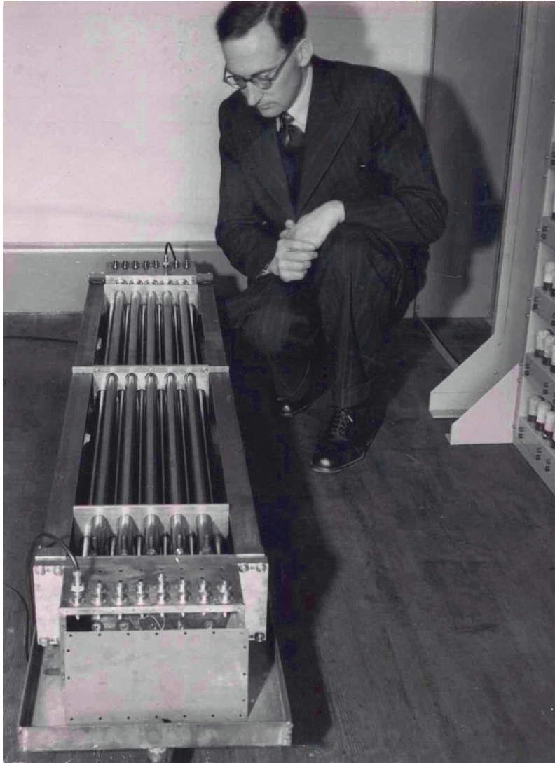
Figure 8.3 Maurice Wilkes with an EDSAC mercury delay line. (Copyright Computer Laboratory, University of Cambridge. Reproduced by permission under the Creative Commons Attribution Licence, photographer: Unknown, source: http://www.cl.cam.ac.uk/Relics/jpegs/delay_lines.jpg )
